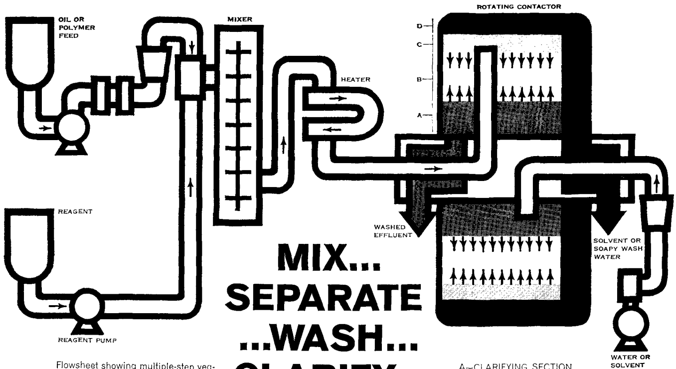
A—CLARIFYING SECTION B—WASHING SECTION C—SEPARATING SECTION D—WITHDRAWING SECTION
